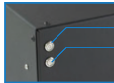
Power on electronic control Enable SSR when safe to engage terminals
